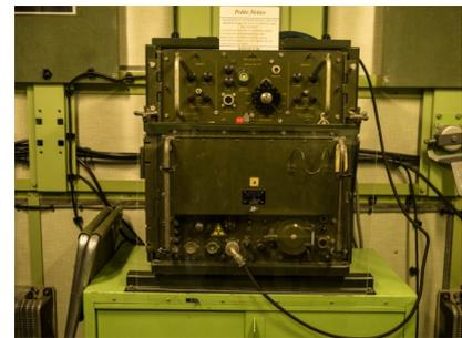
This set was a wideband FM duplex multichannel in frequency range of 50 – 100 Mhz. At first it required the insertion of several crystals, but later it was used with a frequency synthesizer that was developed for the BRUIN Radio Relay
