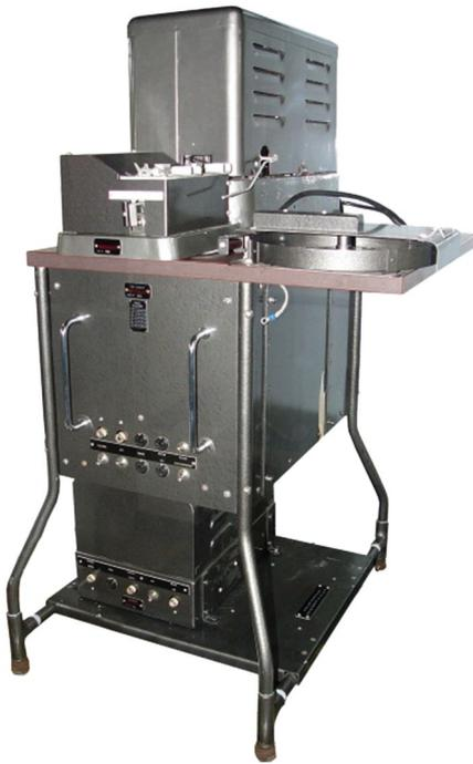
ROCKEX was originally designed and made in a joint venture between the Canadians and USA at the request of the British Government. It first entered service in 1943, but this was an earlier model of the equipment. After WW2 a redesigned model was used to pass Top Secret traffic between the UK and Canada, but in 1955, it was authorised for passing NATO COSMIC Secret traffic.
