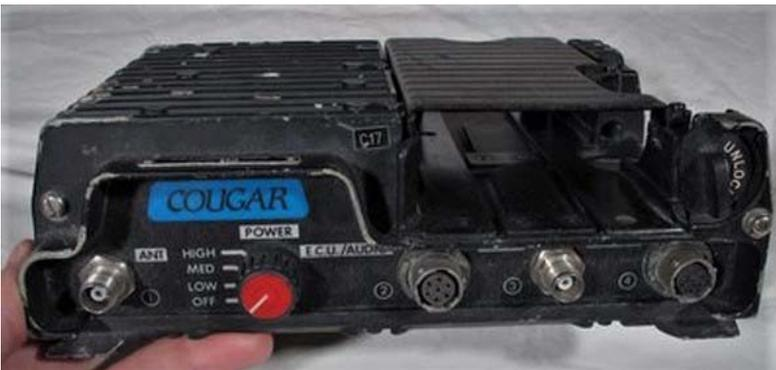
Talk-through radio masts, erected on high spots, were all connected in a single network. It provided mobile access to the radio network wherever the user was; the ops rooms were therefore connected to the soldiers on the ground. The Cougar radio Base Station could be installed in the HQ or in a vehicle - see above. All sets automatically connected to the nearest
