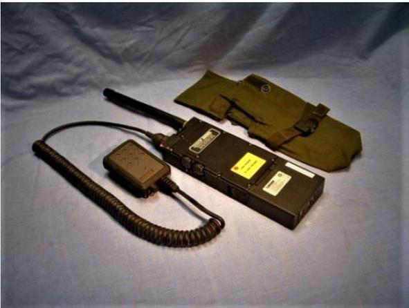
The secure UK/PRC-349, made by RACAL, replaced the non-secure PYE UHF Pocketfone 70 and the PYE Westminster W15 VHF radios that had been introduced in the 1970s. These Pye systems, as explained in a previous object article had suffered from being totally insecure and evidence had shown that all the Pye nets were being monitored constantly by the terrorist organisations.
