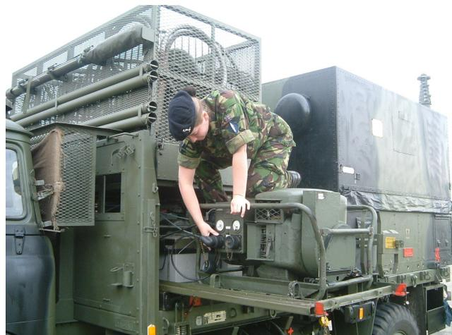
Often Onan comes to mind when power supplies for area communications are mentioned. The AFV 439 has an Onan mounted on the hull to power the C50 Radio Relay. The second is of TRIFFID radio relay, but the PTARMIGAN radio relay was a conversion of the BRUIN/TRIFFID UK/PTC-471. As can be seen the installation comprises of a pallet mounted generator on a 4-Tonne Bedford MK flat-bed.
