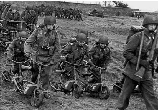
litres. The estimated range was a maximum of 90 miles (140K) at an average speed of 30MPH. It was designed to be packed into a standard parachute container from which it could be unpacked and made ready in 11 seconds. The main problem of this bike was with the container. As the bike only weighed 32 Kg the container fell to the ground at a different speed to the soldier parachuting. It therefore frequently was separated some distance
